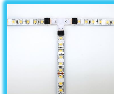
2 - Slide LED strip & T-Strip Connector into each end of Beetle Clip & compress firmly with pliers
